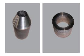
**Die**, **Nipple** (Wire guide) and **Cartridge** are other essential parts of lead extrusion process.
