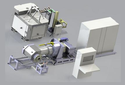
A **Continuous Lead Extruder** consists of several main components/units that are inter-connectable . These parts are mainly, Base frame, Gear Box, Die Block and Die Block tools such as Cartridge, Die and Nipple (Wire Guide), Screw and Screw housing, Thrust bearing assembly, Cooling system, feed pipe system, Melting pots and lead ingots delivery system and finally automatic computer control system.
