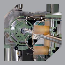
• The process involves many parameters such as friction, metallurgical, extrusion tools design and selection like Die - Nipple, temperature and speed parameters .....
