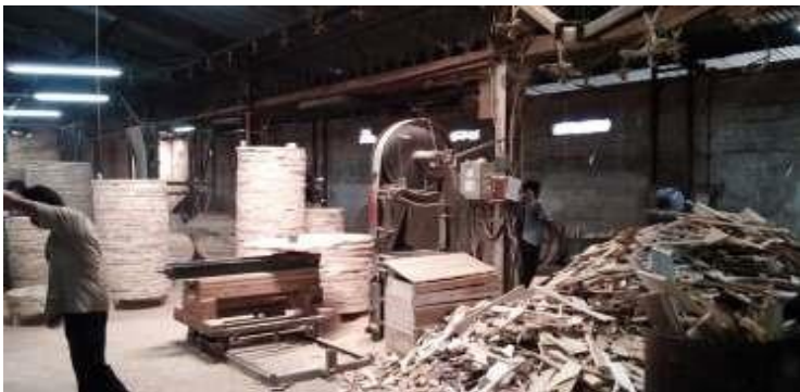
Work in progress: Wood is assembled and cut to round shape.
