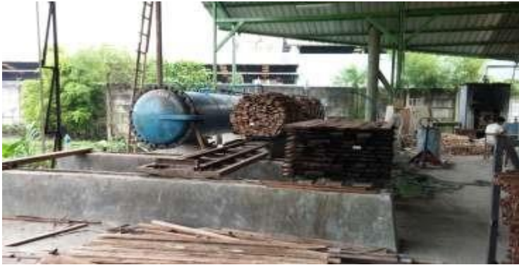
Vacuum Process: Wood is treated with Chemical at high pressure.
